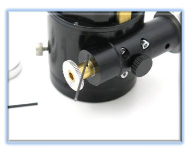
IMPORTANT: Tighten this setscrew securely to avoid backlash introduced by a loose fitting gear.
