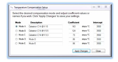
controller will automatically adjust the focus for changing temperatures.
