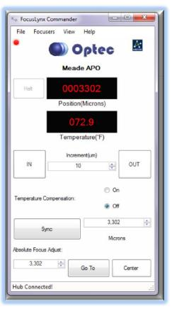
Position value in setup to allow more steps for full travel. Click File- Step Size Wizard in FocusLynx Commander to determine the exact step size and MaxStep values for your focuser and motor.
