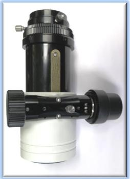
You will use this threaded hole to secure one side of the DirectSync APO silver bracket to the pinion block.
