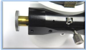
Adjust the gear position so the hub setscrew can be tightened. Insert the 1/16" hex key into the access port to tighten the gear to the pinion shaft. Be sure it is fully secured before continuing. Test the focuser function by moving the coarse and fine focus knobs on the right side of the focuser up and down ensuring smooth free movement.
