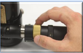
**Step 5**Roll the motor cover up to engage the motor assembly.
