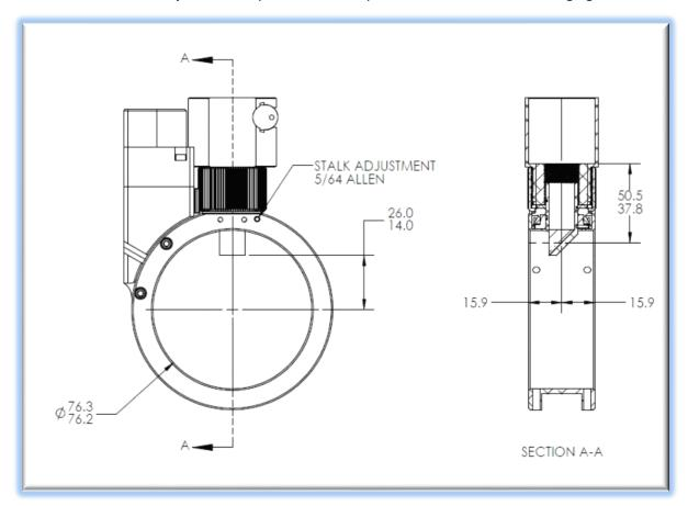
Additionally, the Sagitta focus mechanism provides another 12.7mm of adjustment. Measured from the center of the pick-off prism, this distance ranges from 37.8mm to 50.5mm when the pick-off prism stalk is all the way up (26mm from the telescope optical axis). To calculate the OPL from the reference point, we will add 15.9mm (distance from the reference surface to the center of the pick-off prism) plus any extension of the pick-off stalk.
