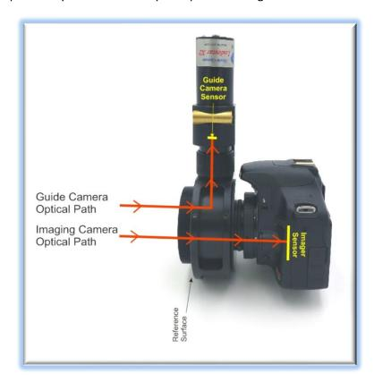
Thus, a camera with a mechanical flange back-focus distance of 17mm plus a 20mm thick filter wheel attached directly to the camera face will have an OPL of 38mm (17mm + 20mm + 1mm for the filters). Ideally, we want our auto-guider OPL to match this distance.
